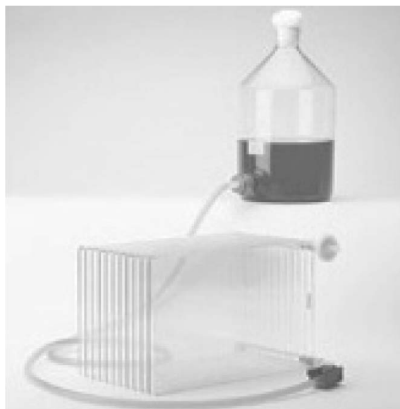
Fig. 1.10 Turn Cell Factory on its side. Raise aspirator bottle above Cell Factory level.
