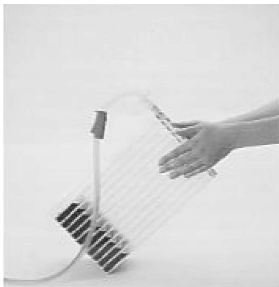
Fig. 1.14 Place the Cell Factory in a horizontal position.
