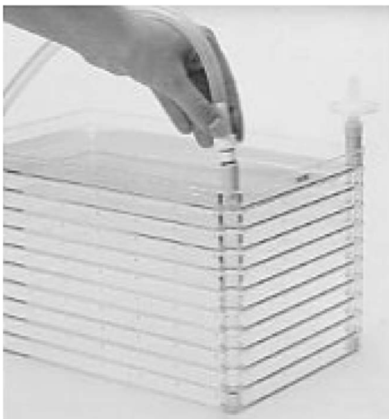
Fig. 1.9 Insert the tube connector.
