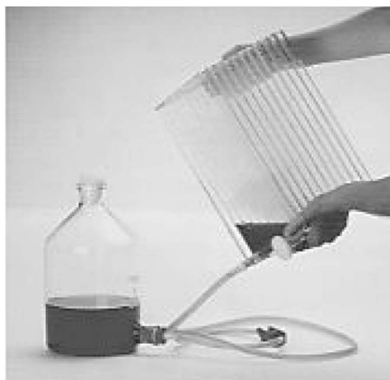
Fig. 1.17 Tilt the Cell Factory to drain completely.
