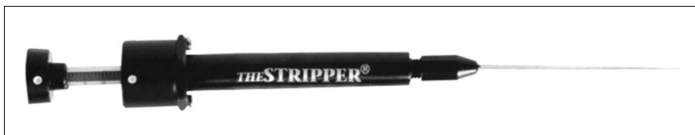
Figure 1A.2.6 The Stripper micropipettor with tip used for manipulating embryonic cells.
